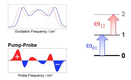
Pump-probe spectra provides more structural information by measuring the anharmonicity of the vibrational potential
