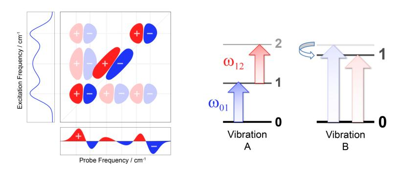
2D IR provides the pump-probe spectrum as a function of the excitation frequency, improving the spectral separation between peaks
