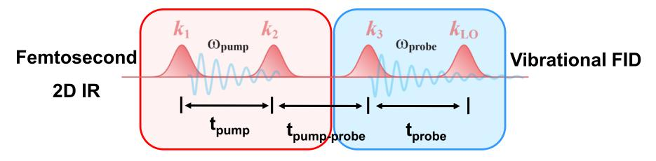
k1 & k2 generated from a single pulse by **pulse shaper**
