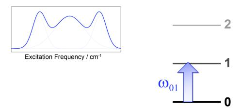
Linear IR spectra measure ground-state vibrational frequencies (peak maxima) and distributions (linewidths)
