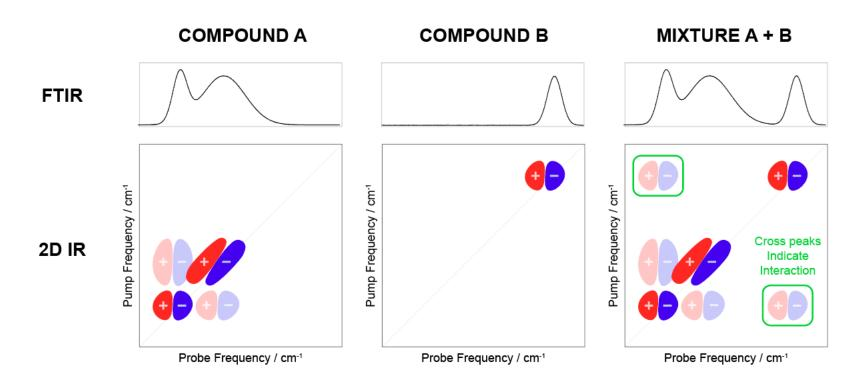
Interactions between two vibrations can also create frequency or linewidth changes in FTIR spectra, but generally these changes will be small and not nearly as direct as the presence of a cross peak.
