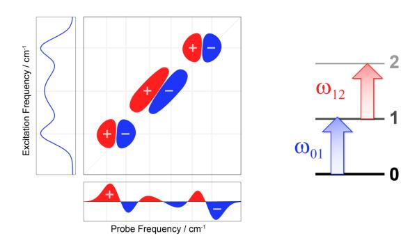
2D IR provides the pump-probe spectrum as a function of the excitation frequency, improving the spectral separation between peaks
